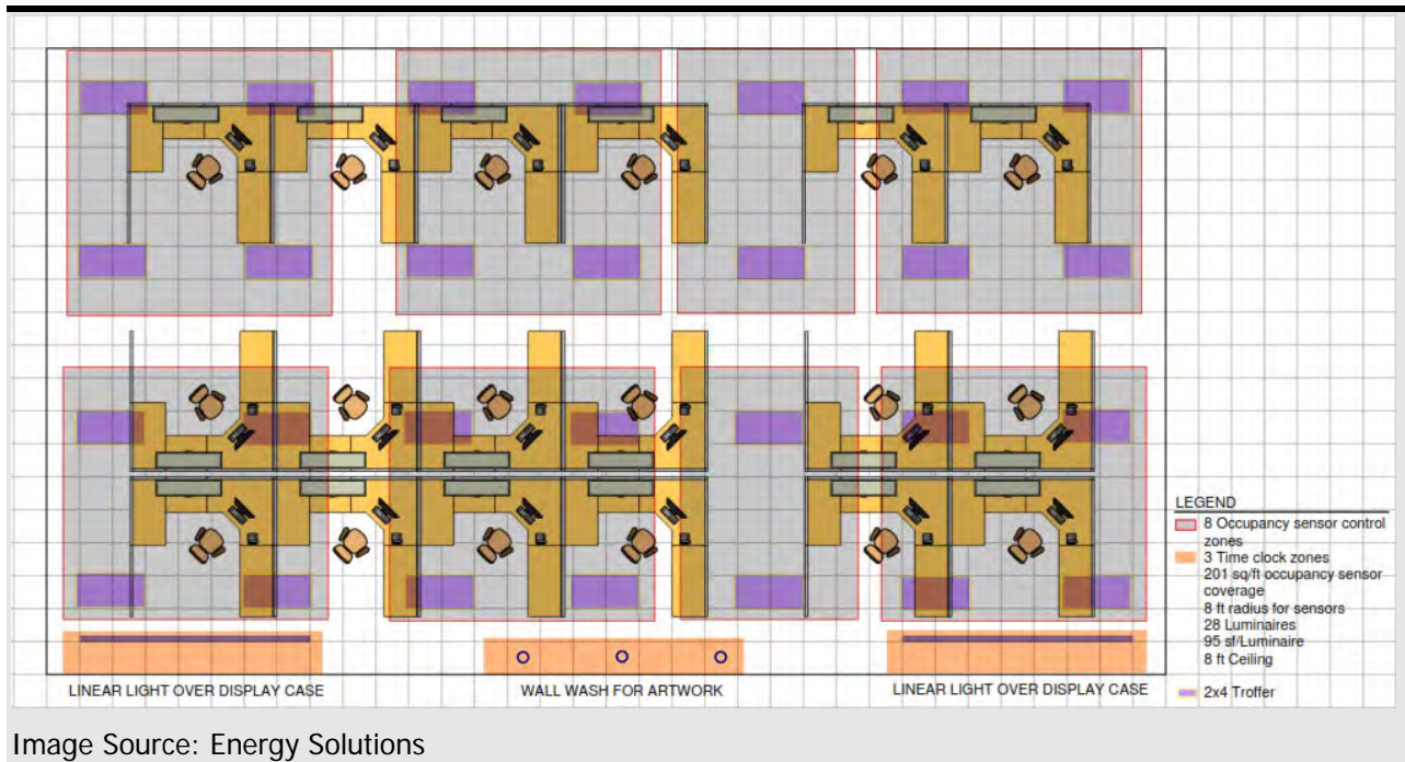
Figure 5-9 (for Example 5-5) An Office Plan With Occupant Sensing Control Zone Layout
