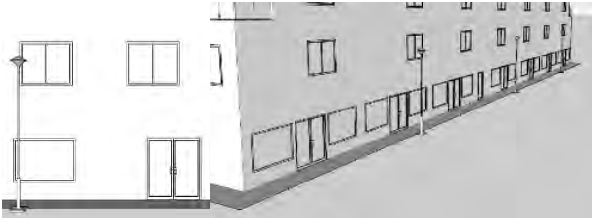
Figure 79: Outdoor Lighting for CASE Example 2: Sideview of an Outdoor Luminaire at the Multifamily Building Site (top left); Outdoor Luminaires for Walkway Lighting (top right); Outdoor Luminaires for Courtyard Lighting (bottom)
