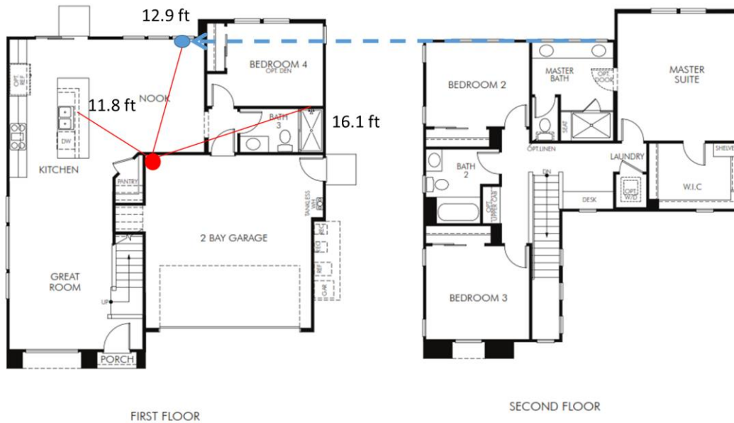
Figure 5-14: Weighted Distance Calculation for the 1,814 Plan with a Centrally Located Water Heater
